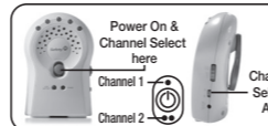
5 Turn Parent Unit on. Slide Power/Channel switch to desired channel selection on front and side A/B button. Power On Indicator will illuminate. Make sure volume is turned down to avoid squealing.
