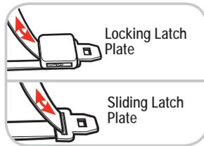
If the latch plate does not slide up and down the vehicle belt, you have a locking latch plate. You should not need to use a locking clip.
