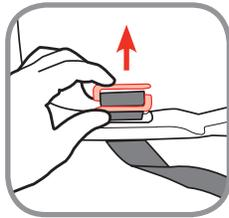
**3. Pull "S" Clip and LATCH Strap Out of Slots in Shell**
