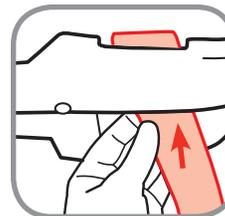
**10. Thread LATCH Belts into Slots on Opposite Side of Vehicle Belt Loops**
