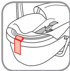
**5. Pull Harness Strap Tight So Adjustment Slides Are Flush Against the Shell**
