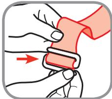
**b.** Slide LATCH belt loop back across "S" clip until LATCH belt loop is centered, making sure top and bottom bar is on the outside of the LATCH belt loop.
