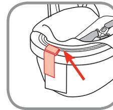
1. Locate Harness Strap Adjustment Slides Under the Pad
