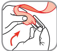
**a.** Slide LATCH belt loop across the "S" clip until it bunches up on "S" clip and the top bar of "S" clip is free from the LATCH belt loop.
